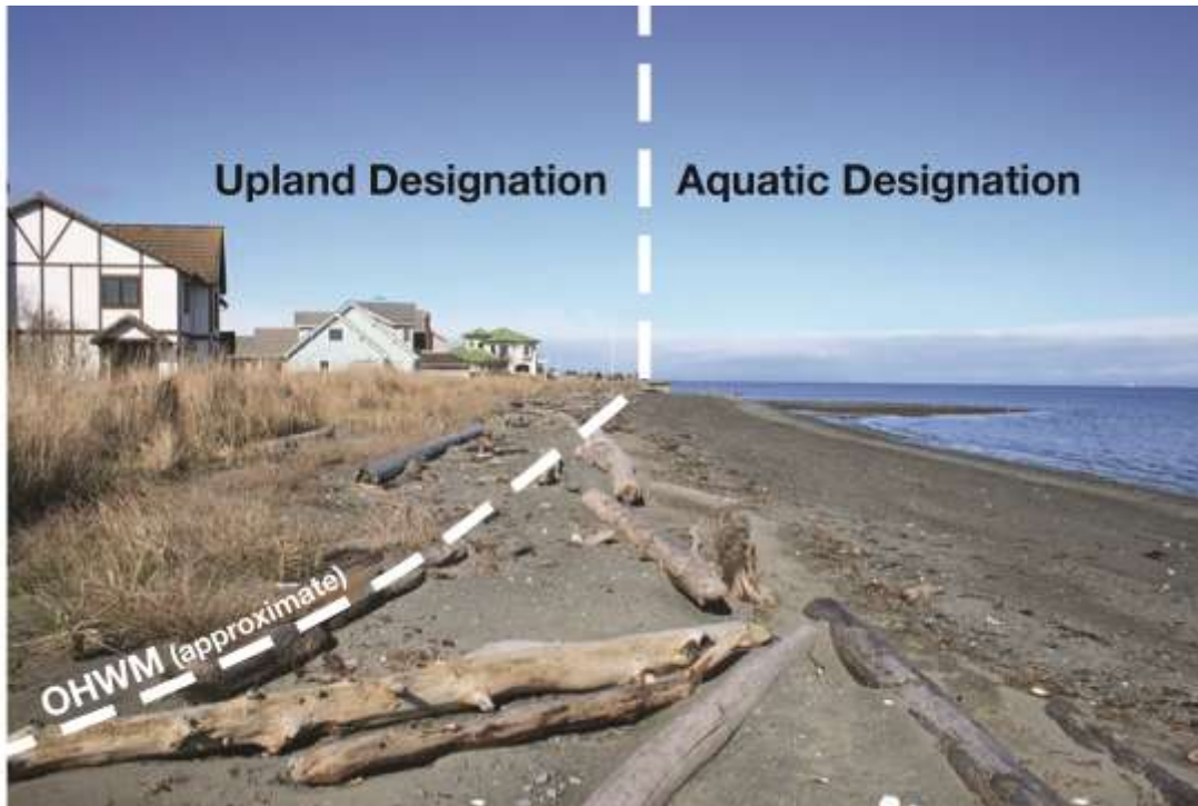
Figure 2-1. Juxtaposition of the Aquatic and upland (shoreland) designations on a typical waterfront parcel (the location of the OHWM needs to be determined in the field)
