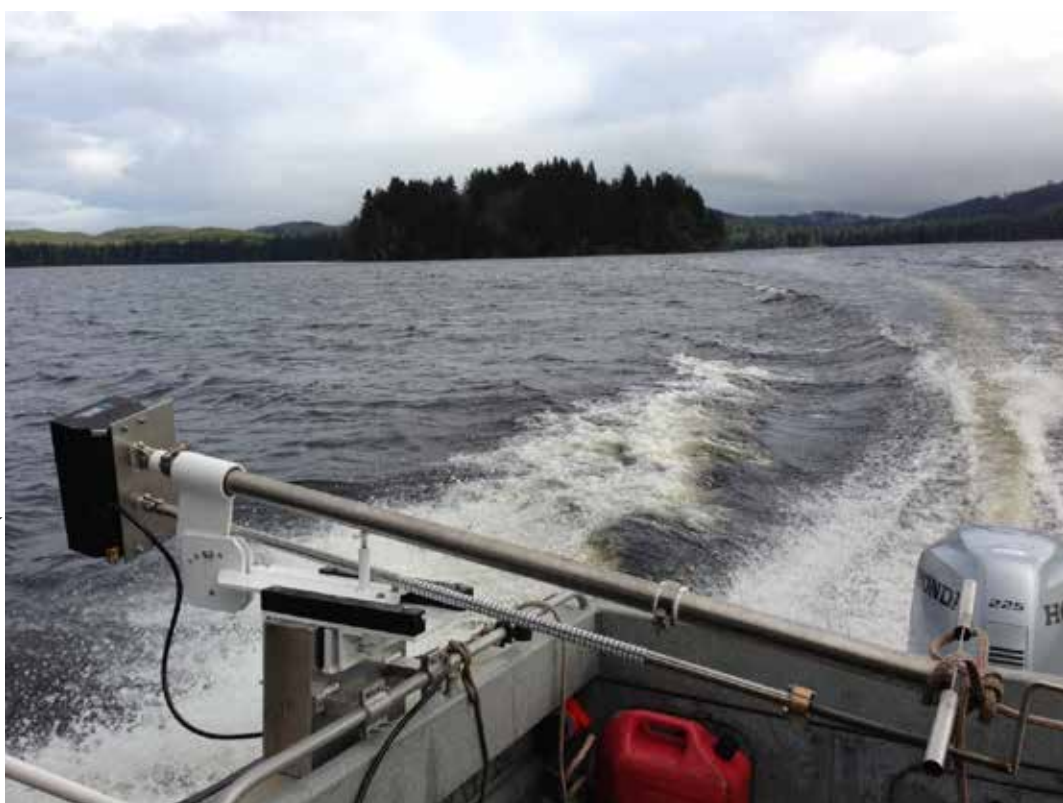
DIDSON mounted to the stern of a borrowed NOAA research vessel during testing in Lake Ozette. Photo: Kim Clark
