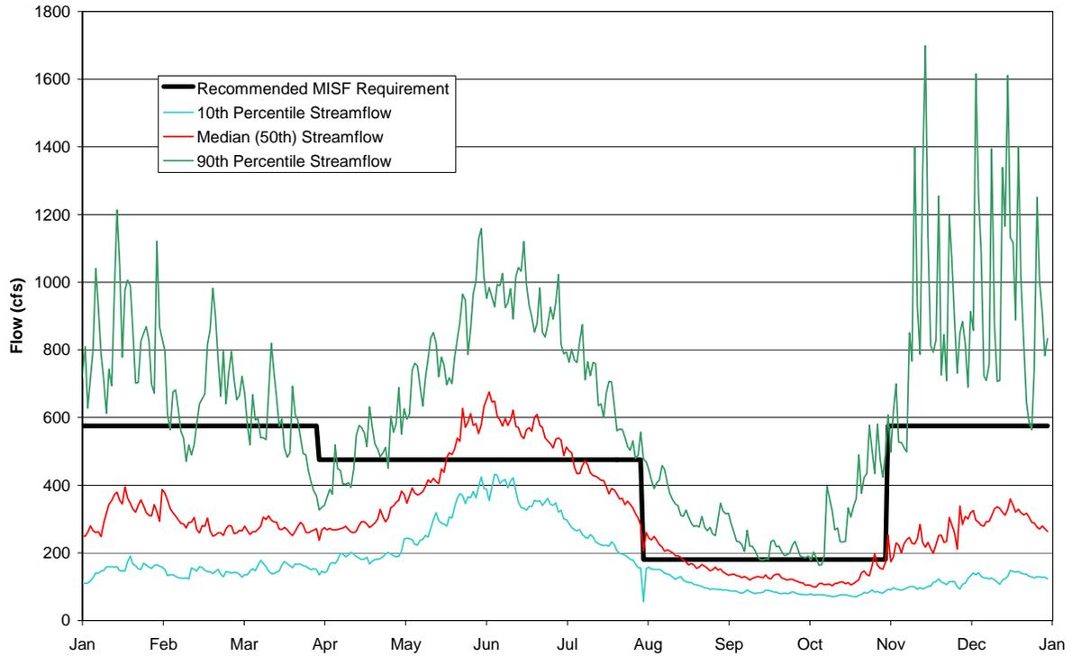
**Figure 1. Synthetic Daily Flow Exceedance Probabilities at the Schoolhouse Bridge Gage (RM 0.75) based on 1970-2004 USGS Streamflow Record and Half Buildout Conservation Plan Assumptions.**
